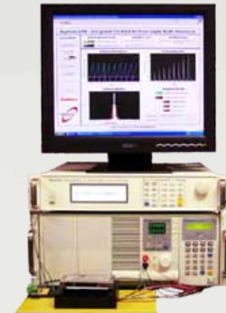
Integrated HW & SW Test Bench for Power Supply Health Assessment
